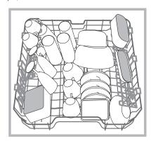
Several dishwasher models are fitted with tip-up sectors\*. They can be used in a vertical position when arranging tea/ dessert saucers or in a lower position to load bowls and food containers
